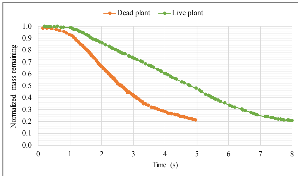
Figure 5-10. Mass loss over time during fast pyrolysis of live and dead inkberry
